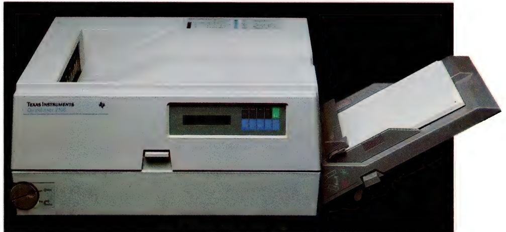
The Omnilaser 2106 from Texas Instruments has a small footprint, weighs only 17 kg, and has enough RAM to print out a full page of graphics – and includes PostScript.
