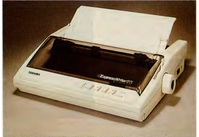
The ExpressWriter 311 has a compartment for storing the power cord, and a carry handle. It can accept font cards, deluded fonts and RAM can be boosted to 48Kb.
